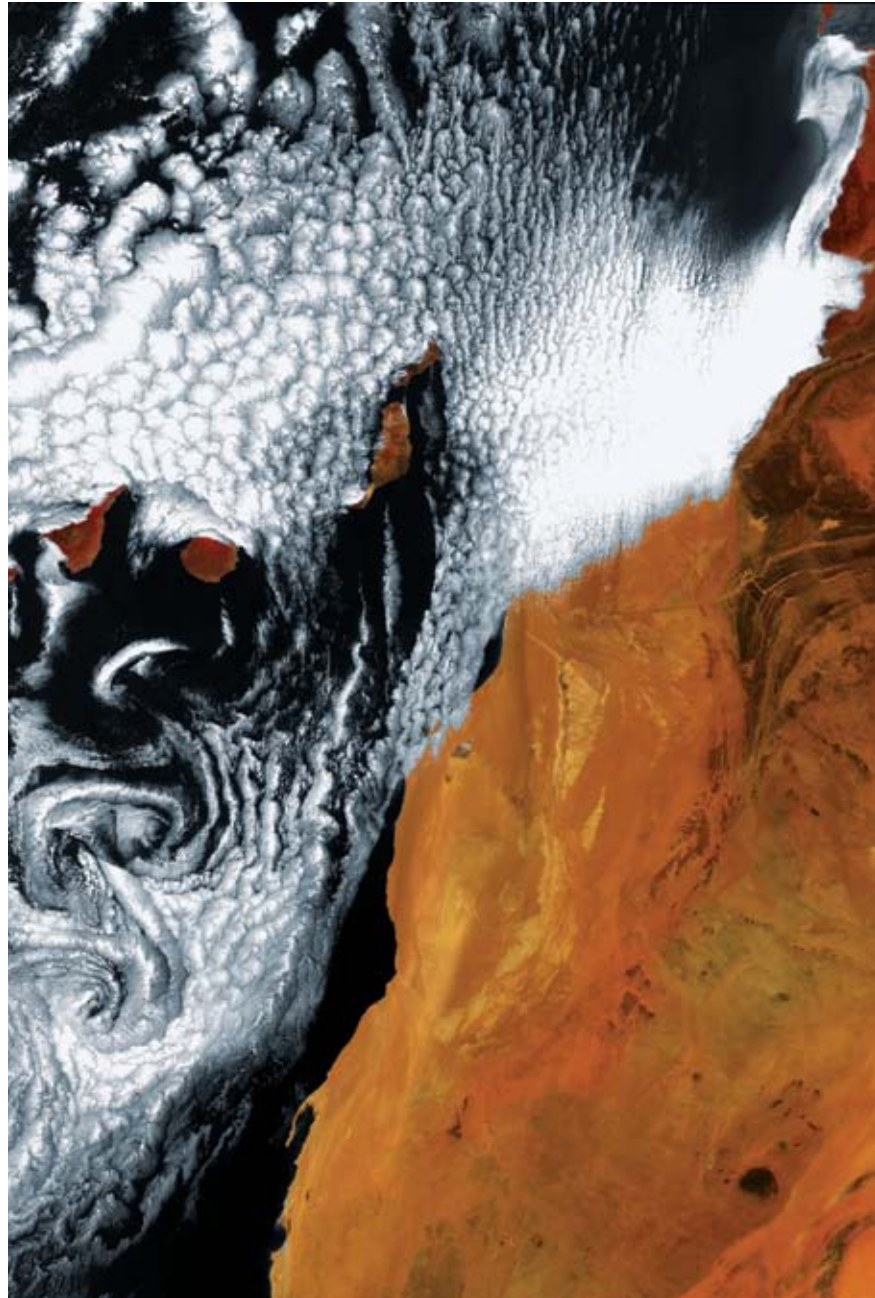
A satellite image of the Canary Islands with unique cloud formations, created by “Von Karman vortices”, off the coast of Africa (right) in the Atlantic Ocean. These vortices, named after aeronautical engineer Theodore von Karman, form as air flows around an object in its path, causing it to separate and create eddies in its wake. The clockwise and counter-clockwise spirals in this image were created as wind blowing from the north over the Atlantic was disturbed by the archipelago. The islands are (left to right): El Hierro, La Palma, La Gomera, Tenerife, Gran Canaria, Fuerteventura and Lanzarote.
