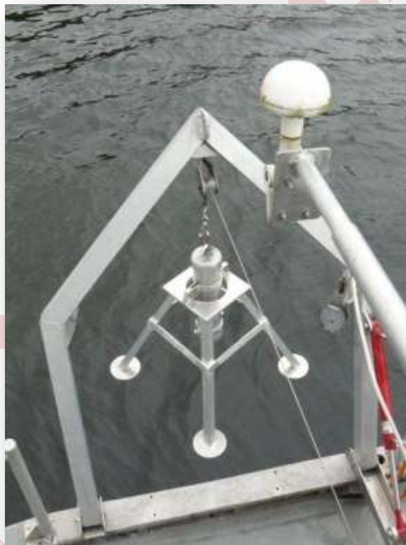
Figure 10. High definition drop camera in the lander frame.
