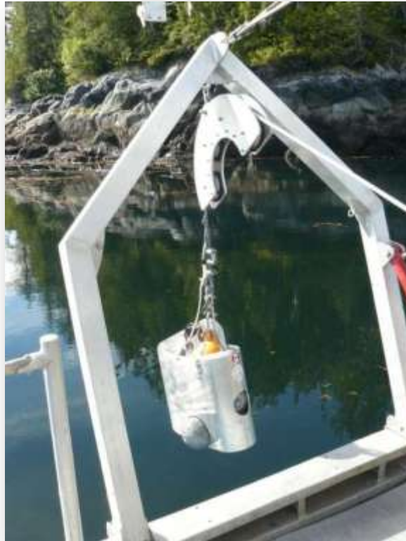
Figure 6. Towed video camera system about to be deployed.
