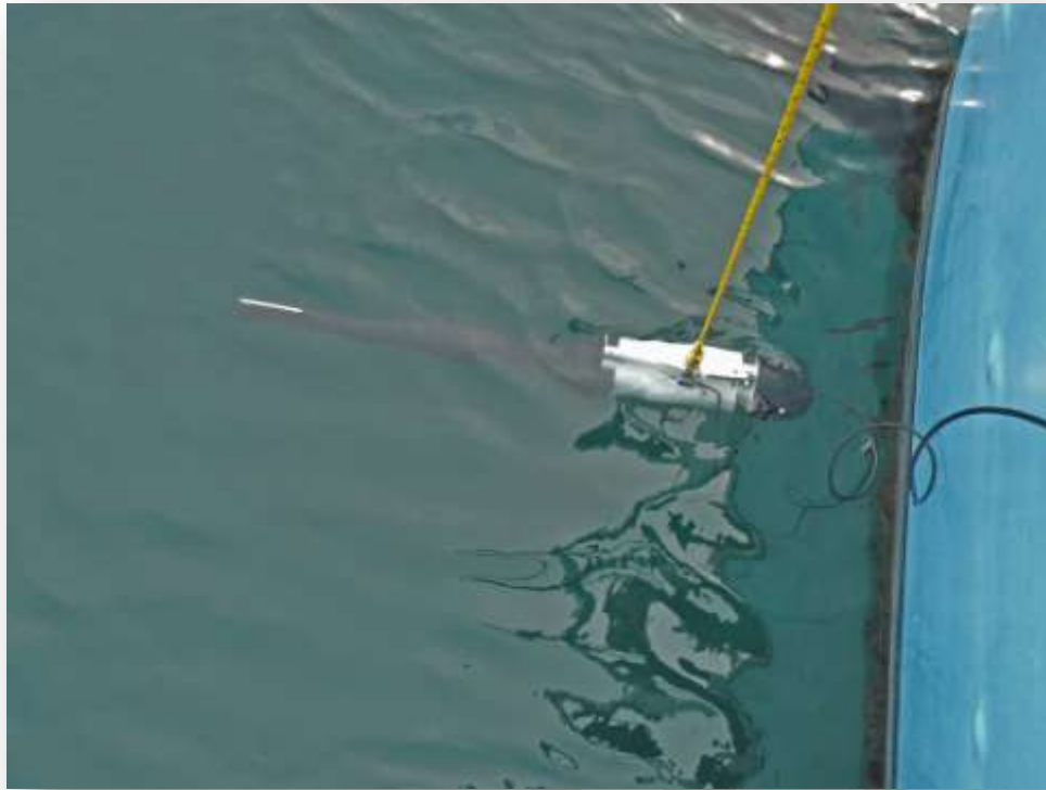
Figure 12. Side scan sonar towfish in towing position.
