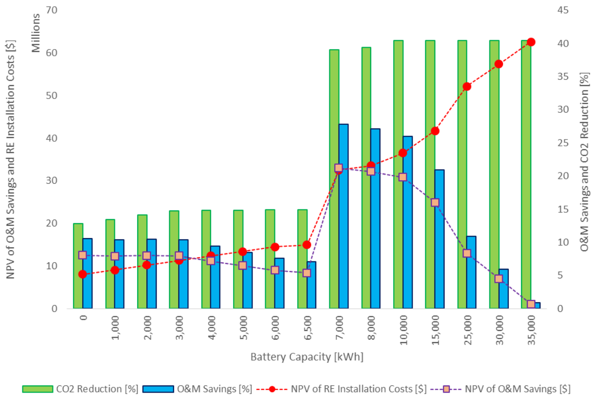
Figure 23: O&M savings, RE installation costs, and CO 2 reductions versus battery capacity for Rankin Inlet, Nunavut.
