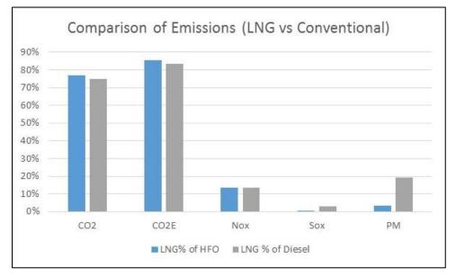
Figure 12: Comparison of Emissions; LNG vs conventional fuels
