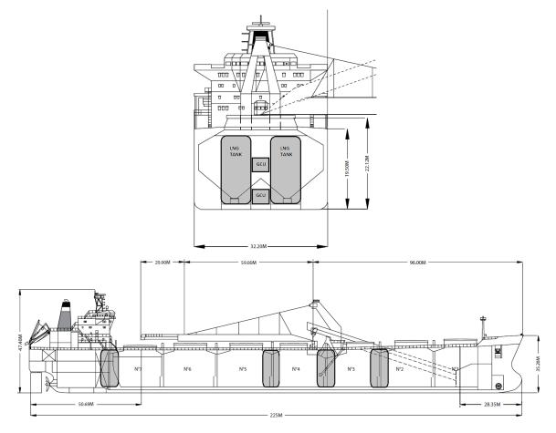
Figure 9: LNG Tank arrangement
