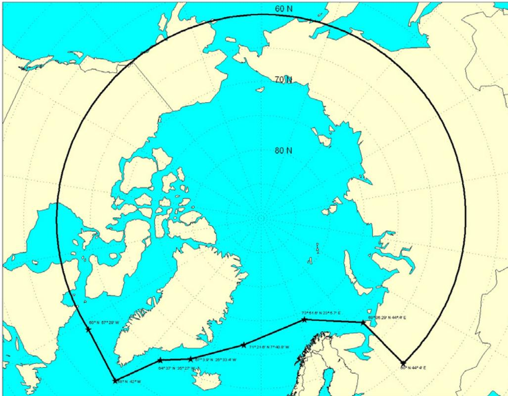
Figure 2: Maximum extent of Arctic waters application. From IMO guidelines for ships operating in polar waters, 2010. Guide section, p 9. Retrieved from [http://www.imo.org/blast/blastDataHelper.asp?data\\_id=29985&filename=A1024\(26\).pdf](http://www.imo.org/blast/blastDataHelper.asp?data_id=29985&filename=A1024(26).pdf)
